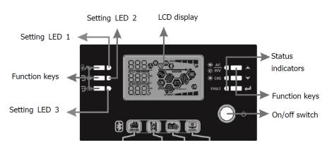
• Press "Up" and "Down" to choose the setting number and press "Enter" to be able to change the parameter, once changed press "Enter" again.
